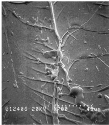
图3 Pd 40 Ni 40 P 20 轴向压缩试样断裂表面的扫描电镜图像 [28] Fig.3 Scanning electron micrograph of the fracture surface of Pd 40 Ni 40 P 20 sample failed in uniaxial compression [28]
